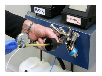
Using the airgun of the unit, remove the remains of water from the outside as well as the paint channel of the spraygun.
