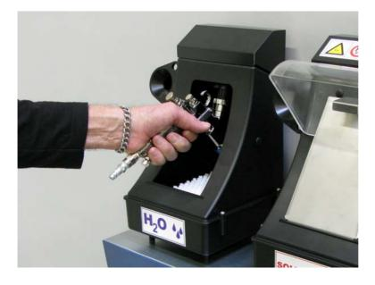
Place the paint channel over the nozzle in the left-hand cleaning box. Press the spraygun up against the nozzle, **and pull the trigger.** Allow the pump to strike 3 strokes.
