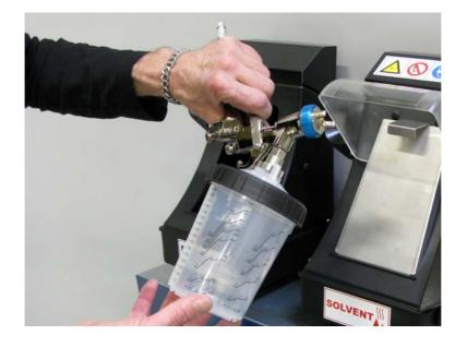
Turn the gun over, pull the trigger to allow the paint to return to the cup.
