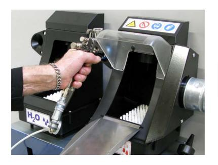
Connect the airline. Blow out excess water through the funnel.
