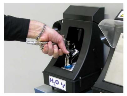
Rub the air-cap of the spraygun against the brush while pulling the trigger.
