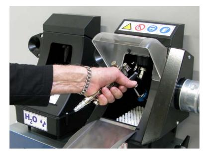
Place the paint channel over the nozzle and pull the trigger. Press the foot-pedal and rinse the paintchannel of the spraygun.
