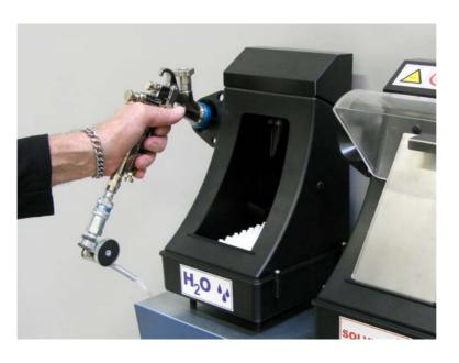
Connect the airline. Blow out excess water through the funnel.
