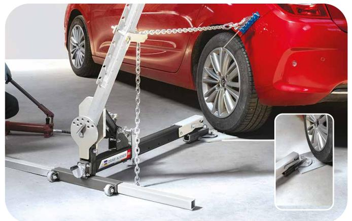
The under-wheel chuck means even quarter-panel damage can be pulled out.
